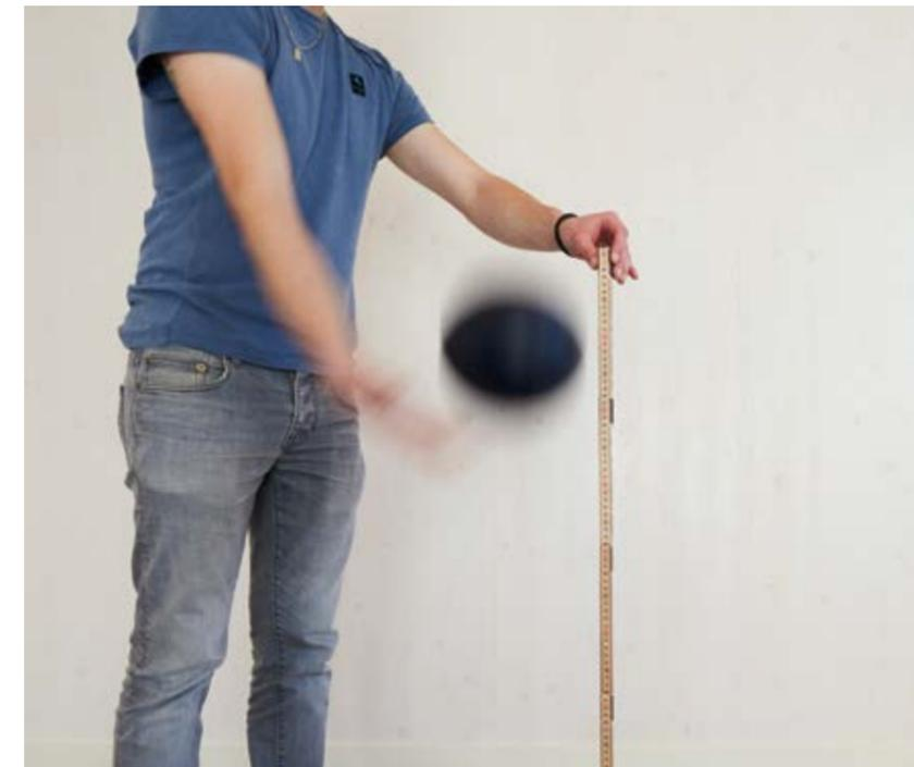
The Japanese rubber ball enables us to make more realistic measurements in the low-frequency range than the tapping machine.
