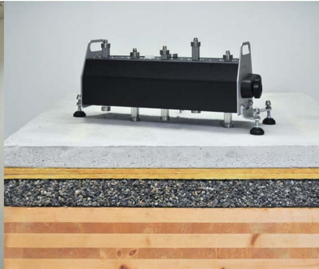
Using the impact sound test bench, pre-test series can be tested efficiently and cost-effectively and ideal structures developed.
