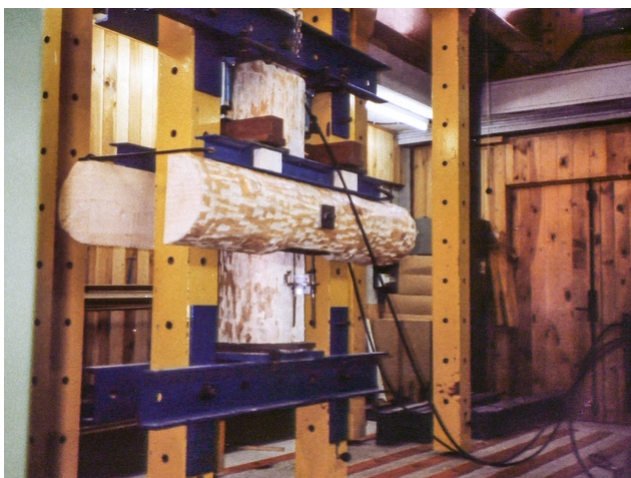
Development and testing of the connection part tong-post...
