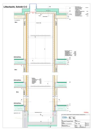
Section through elevator shaft
